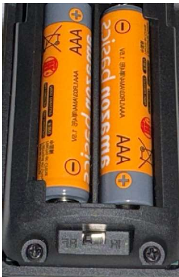
Figure 2 - IR / RF toggle switch - shown here in the RF mode position.
