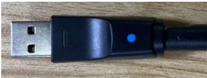
Figure 1 - RF Antenna. Note the blue dot, indicating compatibility with the RC2 remote.
