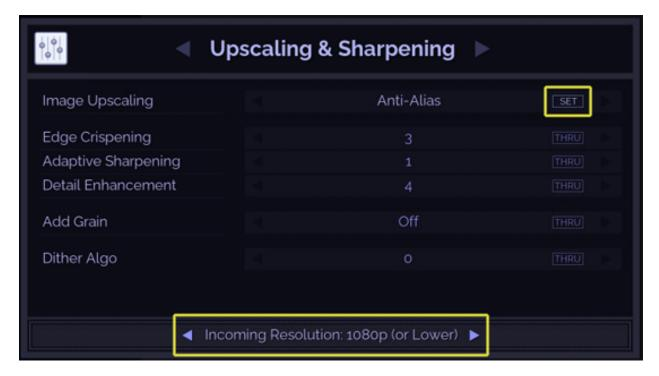
With the Profile Bar set at "Incoming Resolution: 1080p (or Lower)" you will now see the menu page as shown above. This profile appears as a selection in the Profile Bar because we added it in section 3.5.2.
