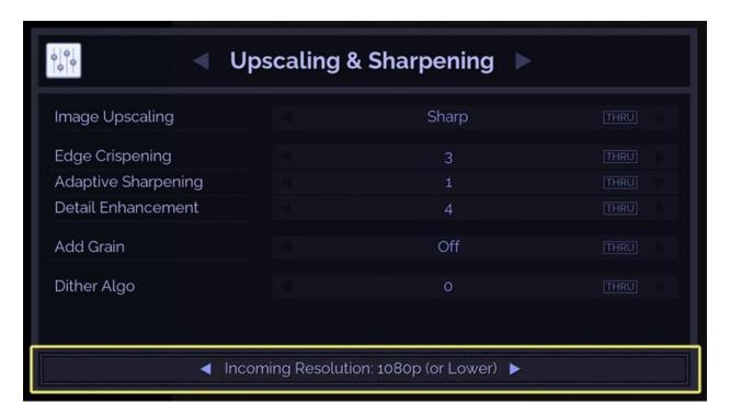
Notice that our new values from above (3, 1, 4) show with the THRU tag. This indicates that the currently selected profile (as shown in the Profile Bar) is not setting these values and these will be unaffected by this profile, if not set here.
