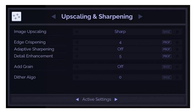
Notice how the Envy has automatically recalled our Upscaling & Sharpening settings for 1080p, and that this shows as our Active Settings. The PROF tags here indicate the settings are coming from an active profile – in this case, the profile we added for 1080p or lower.
