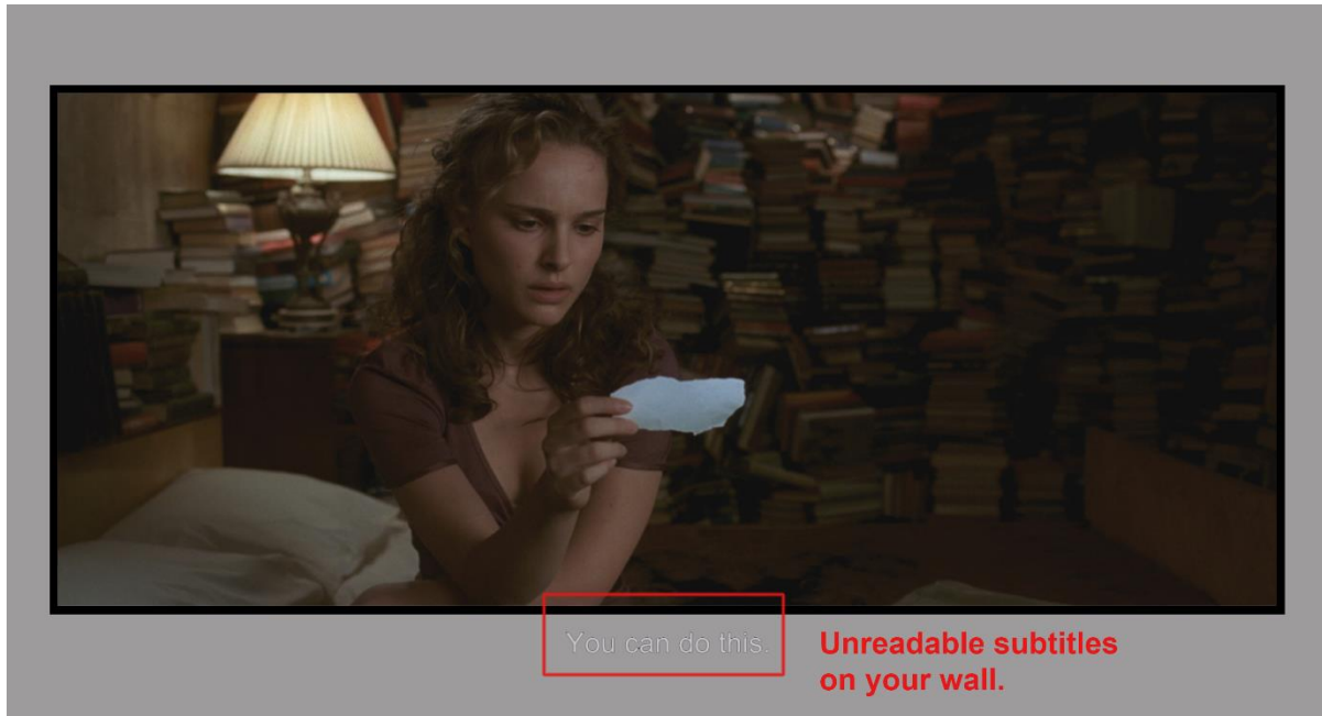
Image 2: With the projector zoomed to fill the screen, there is no zoom left for the subtitles!
