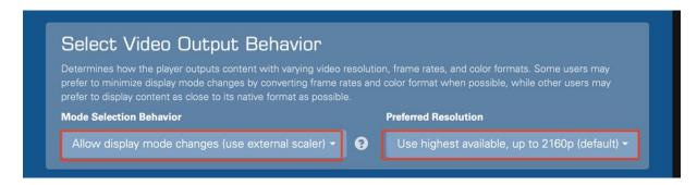
The "Allow display mode changes" option ensures the Kaleidescape outputs the original resolution and framerate of the movie. Otherwise, it will output movies at 60p instead of 24p, which makes HDMI switching faster (and why it is often set up this way), but at the expense of video playback quality. See Appendix A for more information.
